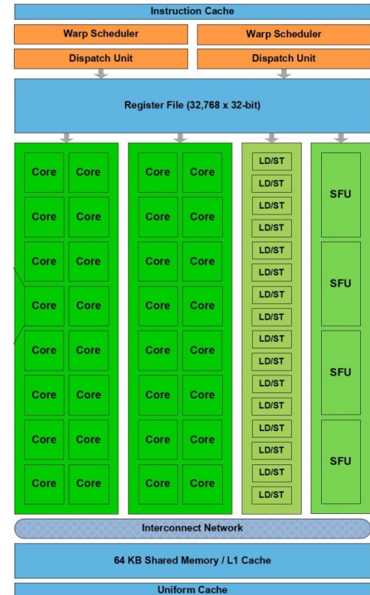
Fermi Streaming Multiprocessor (SM)
